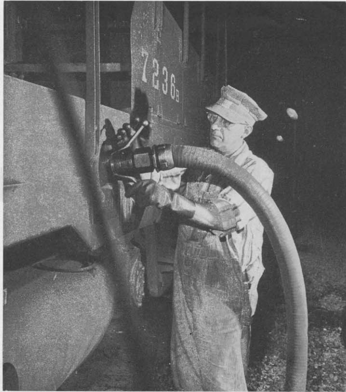
Laborer N. J. Lambert services thirsty diesel at Nelson Rd. fueling station, Columbus.
